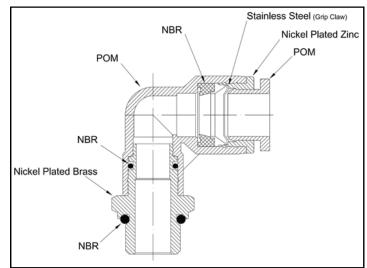
O ring seal on G and TRI Thread Models
